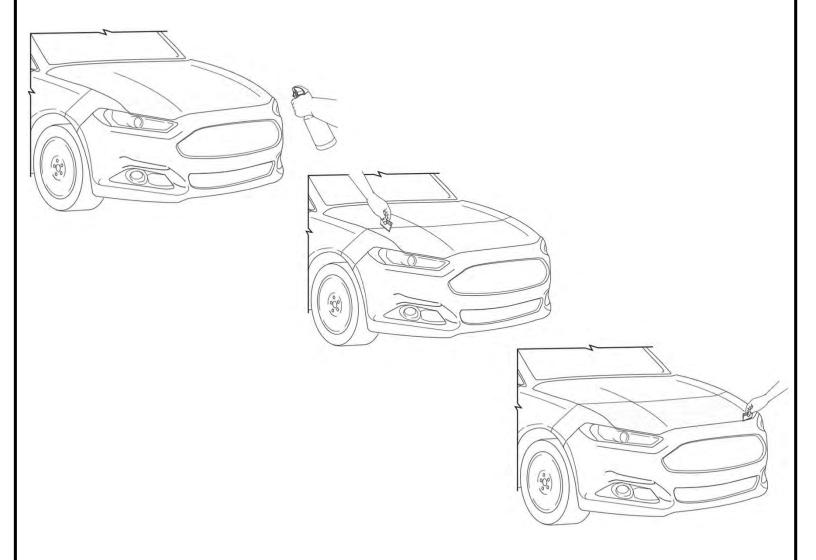
Stretch the film as necessary to align along the edges. Precut patterns account for most "fingers" in the design, so when stretching to align edges, most "fingers" will lay flat on the surface. "Fingers" are localized gaps in the film in aera of high contour. Continue to squeegee out the aid solution towards the edges as you stretch and align the film on the surface.
