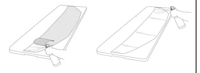
Next, spray mounting solution generously on the area in which Paint Protection Film will be applied. Gently position the film on the surface to be protected while identifying an alignment point such as the center, an emblem or a corner on the surface. This will be the starting point of the wet out.
